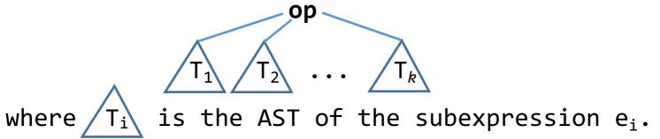
**Note:** ASTs of <u>infix</u> expressions are binary trees, as infix notation doesn't allow operators of arity > 2.
