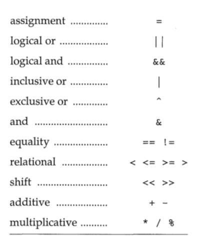
Figure 2.9 A partial table of binary operators in C, in order of increasing precedence; that is, the assignment operator = has the lowest precedence and the multiplicative operators \*, /, and % have the highest precedence. All operators on the same line have the same precedence and associativity. The assignment operator is right associative; all the other operators are left associative.
